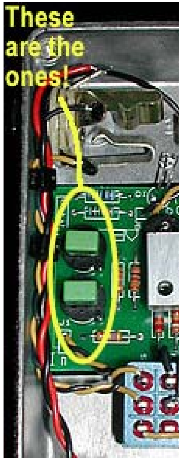
Figure: The two capacitors are housed in sockets as pictured. Use tweezers or pliers to gently remove them. Don’t pull out the black or silver transistor (which is also seated in a black, plastic socket on the other side of the circuit board!).
